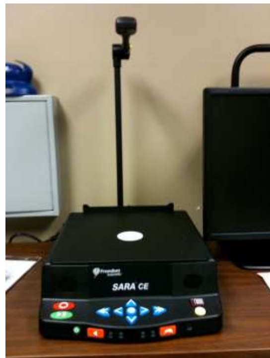
SARA-CE, a device used by the ODS to scan printed materials and convert them into audio files.
