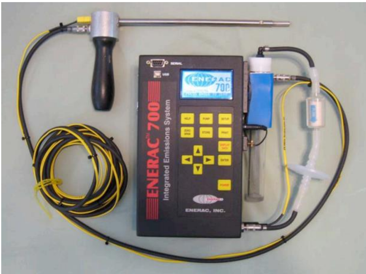
Figure 3-5. Enerac 700 5-Gas Analyzer.
