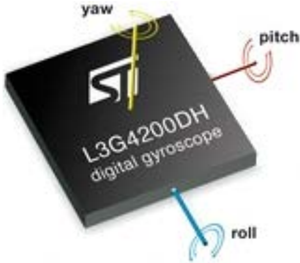
Figure 16. L3G4200DH axis orientation.
