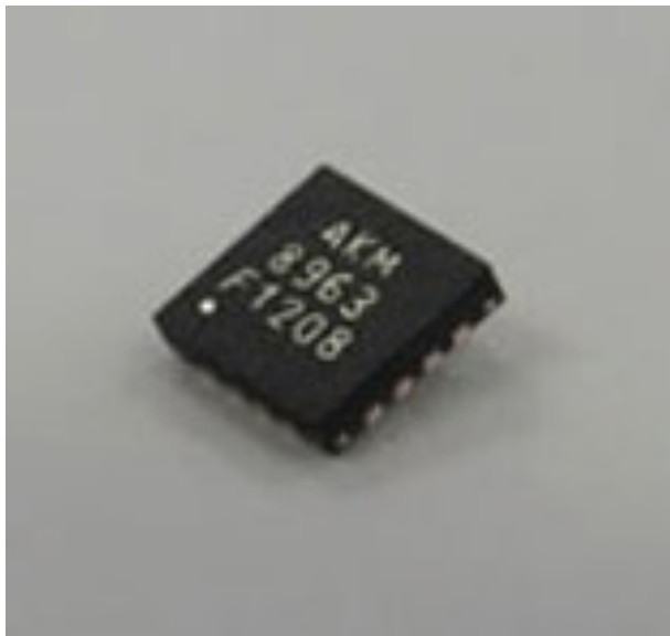
Figure 12. AK8963 digital compass (courtesy of Asahi Kasei Microdevices Corp.).
