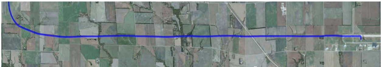
Figure 57. Lateral track during ILS 17 instrument approach, visual
