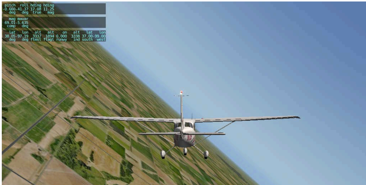
Figure 41. X-Plane model during 45° performance turn.
