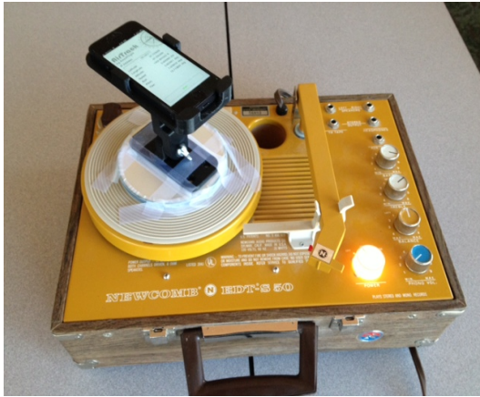
Figure 24. Rotation test about Z-axis.
