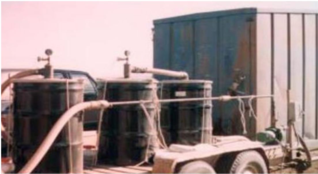
Figure 2.8. Mobile Packed-Bed Adsorption System
