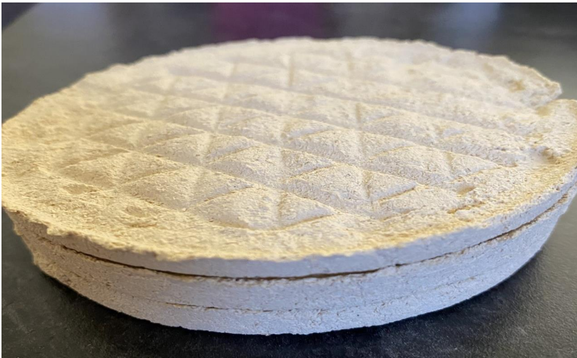
Figure 5.14. Ceramic Samples Subjected to Temperature Range of 850–1200°C
