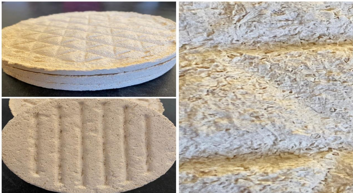
Figure 6.7. Ceramic Filter Surface with 55% Sawdust
