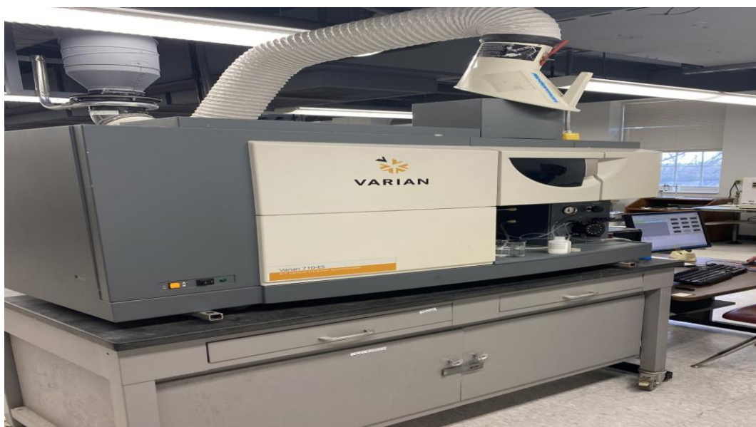
Figure 5.16. Varian 710-ES Optical Emission Spectrometer Testing System
