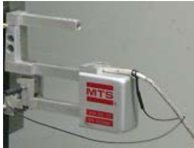
Figure 13 Extensometer: Displacement gage used for old procedure (Courtesy: NIAR)
