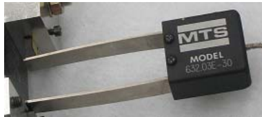
Figure 12 Clip Gage: Displacement gage used for the proposed method (Courtesy: NIAR)
