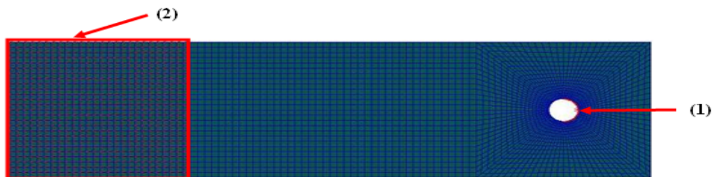
Figure 42 Two dimensional FE model with boundary conditions
