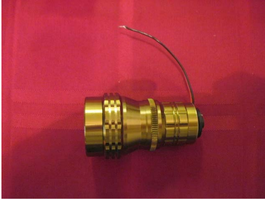
Figure 5: Completely assembled internal laser assembly.
