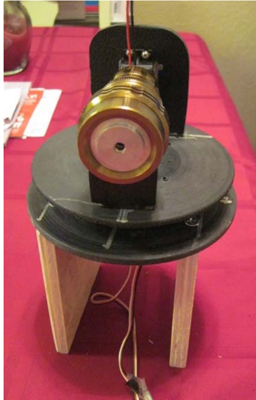
Figure 7: Internal laser assembly attached to control servos, front view.
