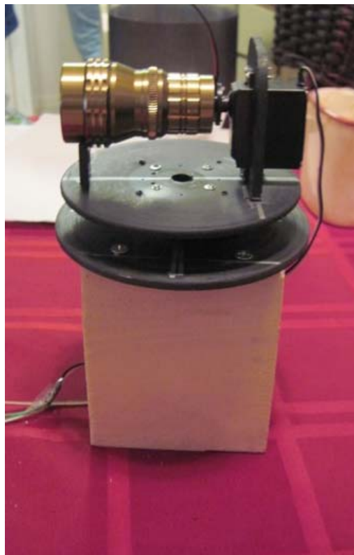
Figure 8: Final internal assembly minus housing, side view.
