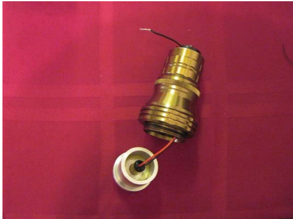
Figure 4: Break down of internal laser assembly, view of laser diode.
