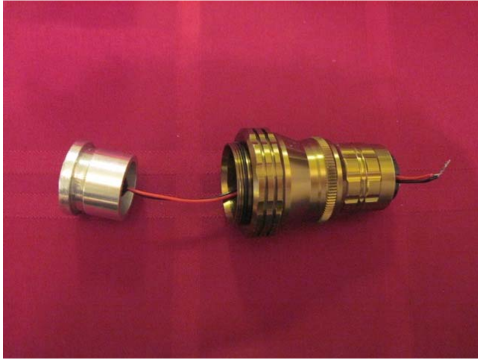
Figure 3: Break down of internal laser assembly.
