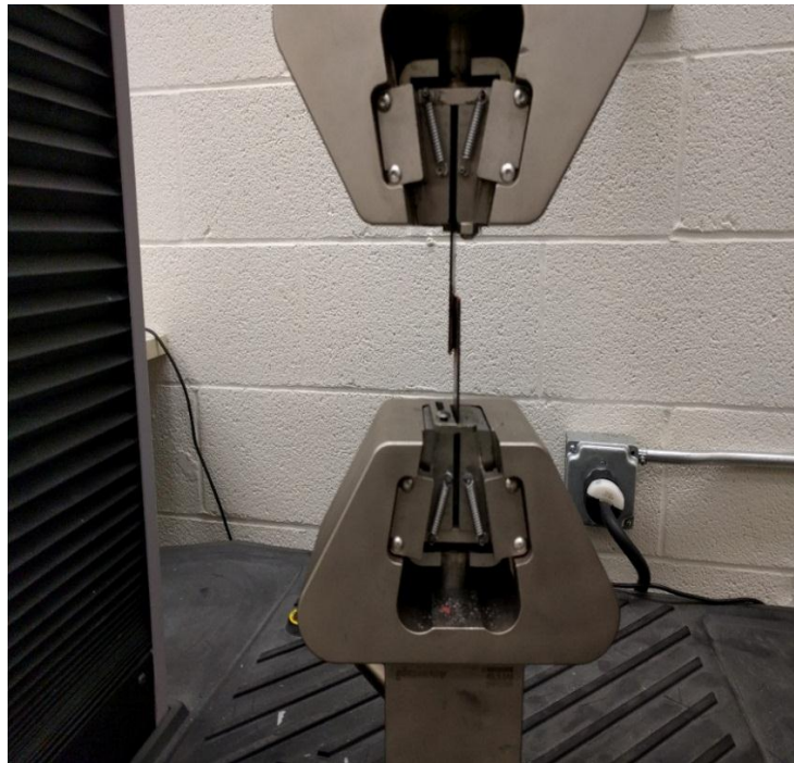
Figure 3.16. Sample placed in MTS tensile testing machine.
