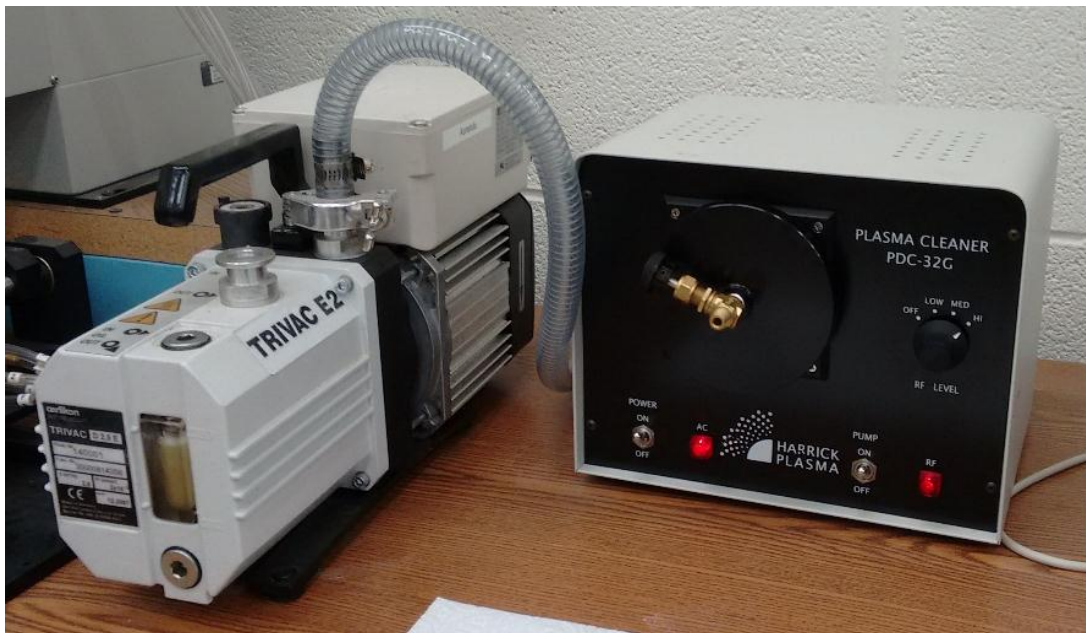
Figure 3.5. Harrick plasma cleaner and vacuum pump.
