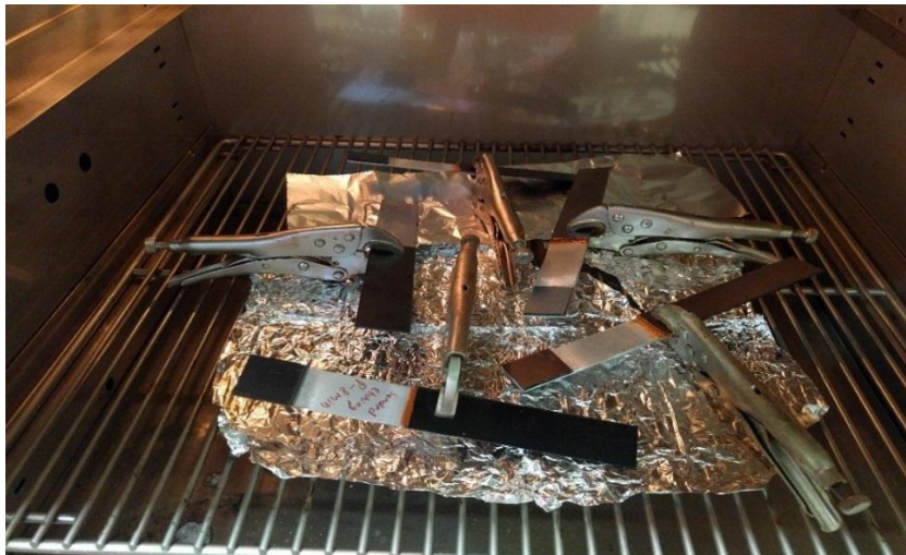
Figure 3.15. Single lap joint specimens prepared and cured in oven.
