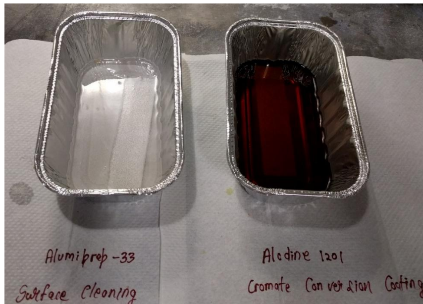
Figure 3.12. Alumiprep 33 (left) and Alodine process (right) carried out simultaneously.
