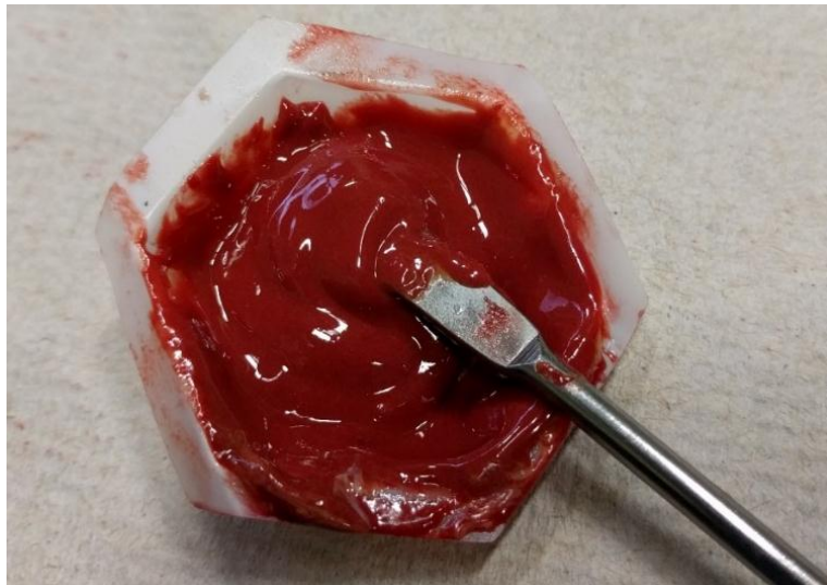
Figure 3.13. Preparation of adhesive mix for bonding.
