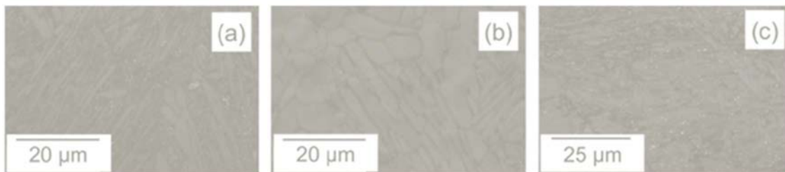
Figure 2. EBSD maps of various microstructures produced by additive manufacturing (a) as build LB-PBF (b) heat treated LB-PBF and (c) DLD (Leuders et al., 2012)
