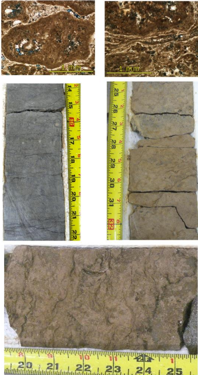
Figure 12: F-3 Bindstone. Microbial in origin and generally found as patch reefs that in core are observed as thin units that interfinger within other units. Occasionally these reefs will grow to dominate an area, which is represented in core with multiple feet of intense microbial fabric within the rock. Thin section images from P13697 at 3525 m (11566 ft.) depth.
