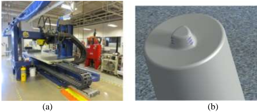
Figure 5.4. Producing FSSW: (a) MTS® gantry machine, and (b) weld tool design used to produce swept FSSW.
