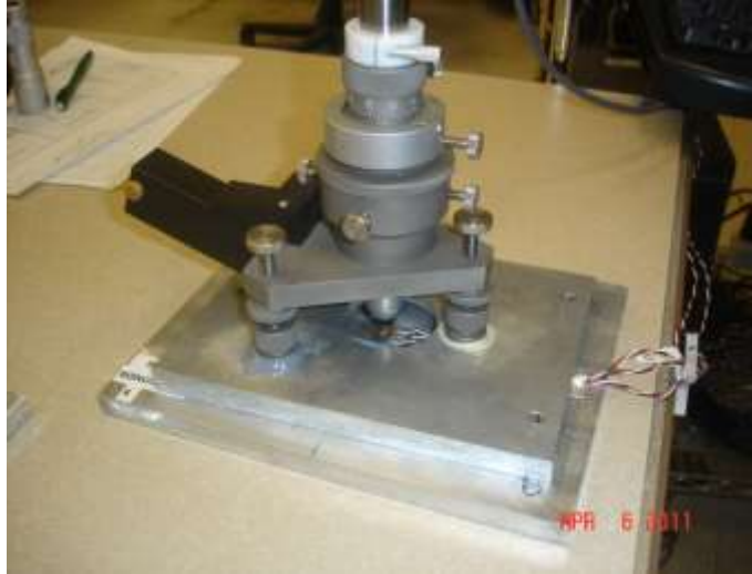
Figure 15 - ASTM E837 Residual Stress Determination Drilling Apparatus
