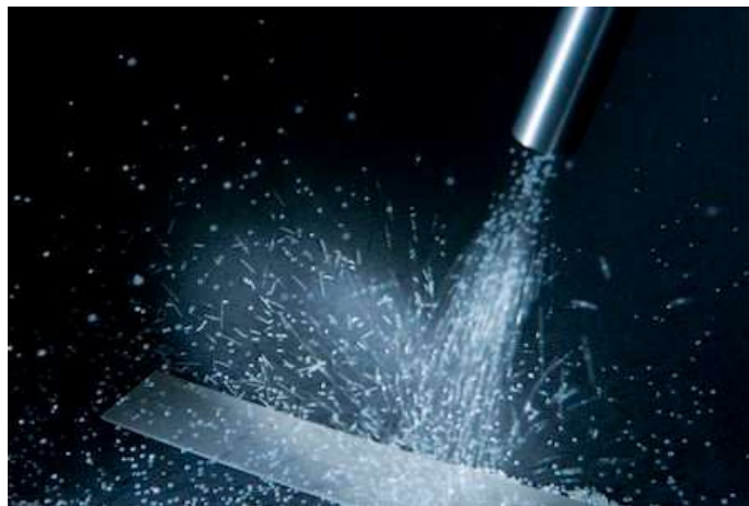
Figure 1 - A shot stream from a nozzle impacts a strip of metal (ceramics.org)
