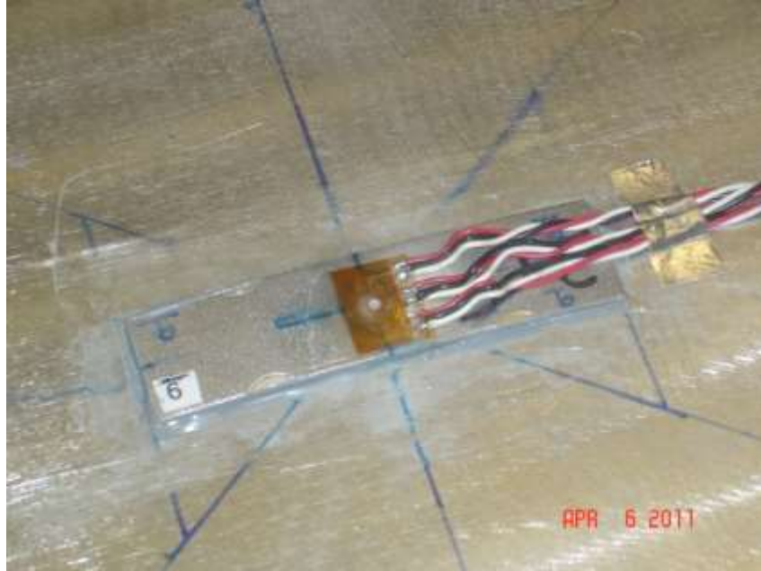
Figure 14 – Three axis strain gauge used to determine strain in the substrate.
