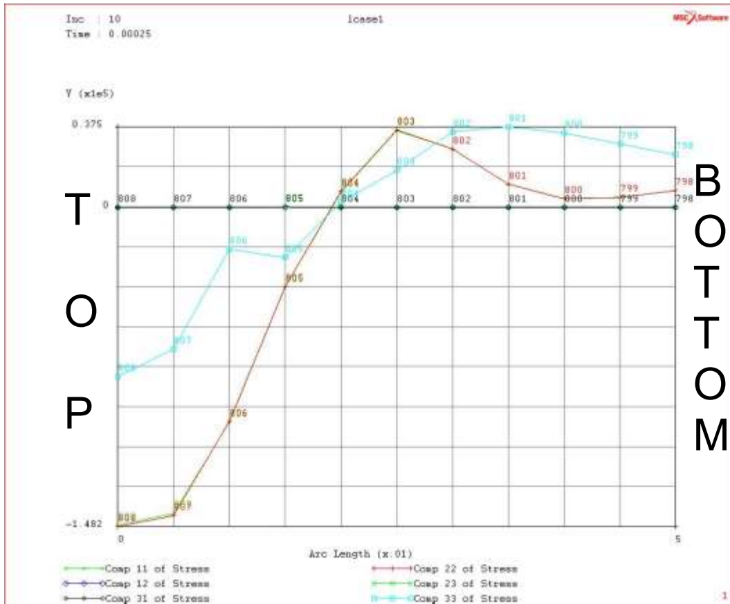
Figure 9 - Graph of the results of the FEA model. Components of the residual stress through the thickness of the part is compressive near the surface and the tensile residual stress deeper below the surface.
