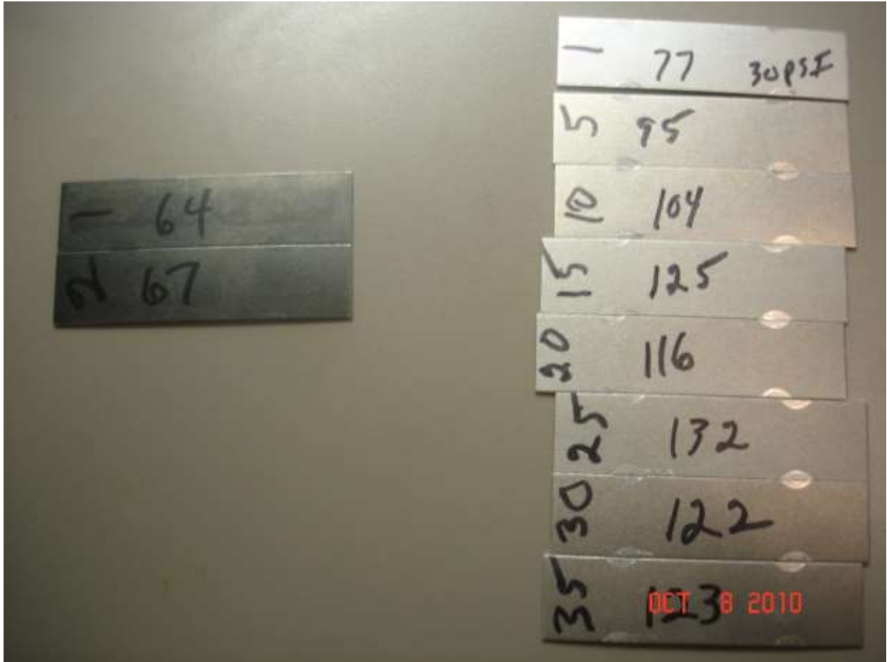
Figure 11 - Steel Almen strips on the left and Aluminum Almen Strips on the right, labeled with exposure time and arc heights measured in ten thousandths of an inch.
