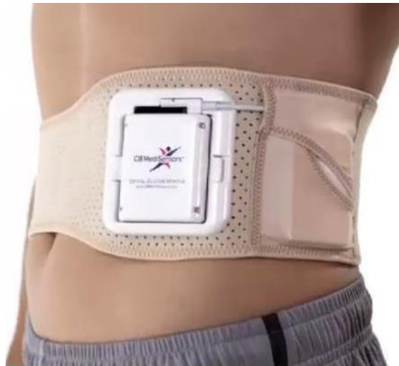
Figure 14. C8 MediSensor using Raman Spectroscopy [24]
