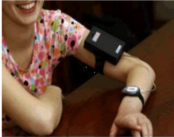
Figure 27. Glucoband using Electromagnetic Sensing [40]
