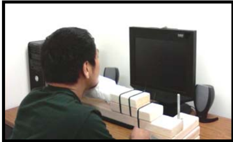
Figure 4.1: Experiment scene setup including Tobii monitor, speakers, keyboard, mouse, and chin rest.
