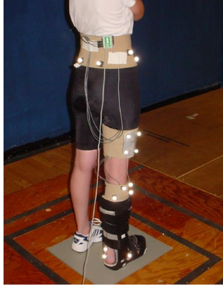
Figure 2.16 Reflective markers placement on lower extremity and pelvis [64].
