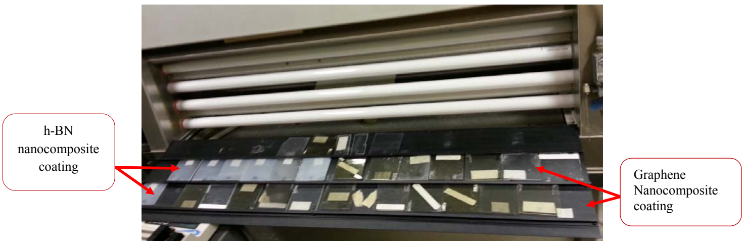
Figure 44: UV Degradation Test Using the QUV Weathering Tester
