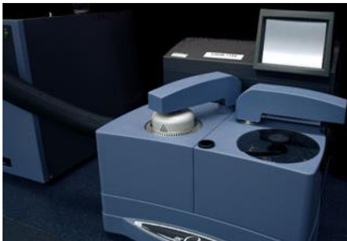
Figure 30: Different Scanning Calorimetry Q-2800
