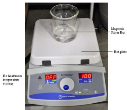
Figure 22: Hot Plate from Fisher Scientific used to mix the Coating System
