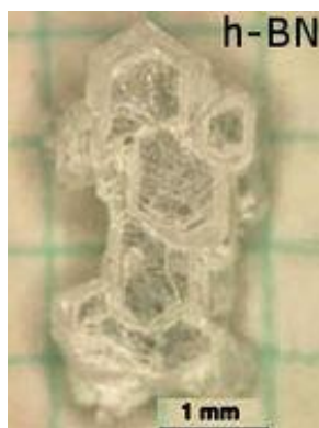
Figure 15: Magnified Sample of Crystalline hexagonal boron nitride
