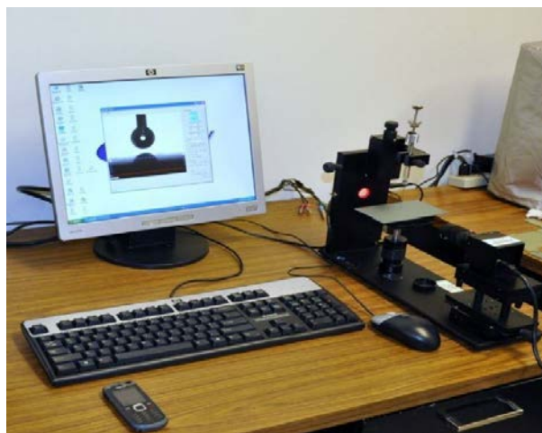
Figure 27: Optical Water Contact Angle Goniometer
