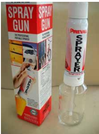
Figure 20: Preval Spray System used to Spray Paint Test Samples
