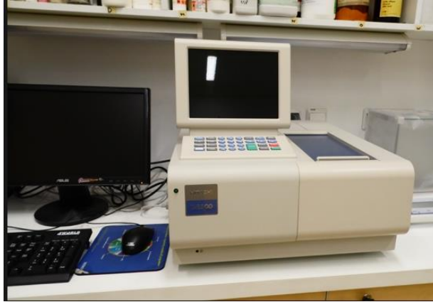
Figure 28: UV-Vis Spectrometers U-2900 Hitachi
