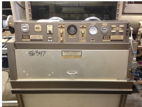
Figure 25: QUV Accelerated Weathering Cabinet used to simulate the Weathering of nanocomposite Coatings
