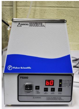
Figure 23: Fisher Scientific FS 200 Sonicator used to Mix the Nanoparticles inside the Coating System
