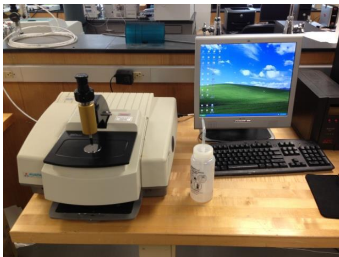
Figure 26: Thermal Nicolet magna 850 IR Spectrometer used to Perform FTIR Studies
