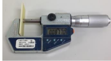
Figure 24: Mitutoyo 293-725 Digimatic Micrometer used to Control the Coating thickness
