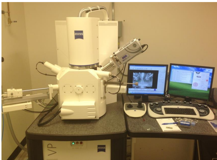
Figure 29: SIGMA Series of Field Emission Scanning Electron Microscope
