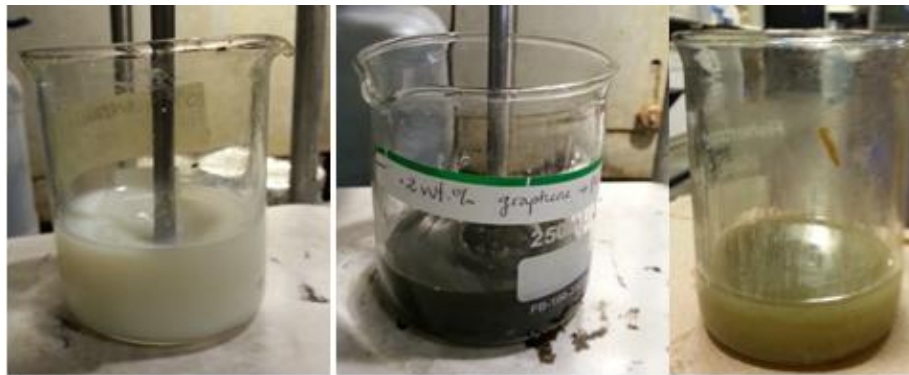
Figure 40: Mixtures of PU & Silanized h-BN (left), PU & Silanized graphene (center), PU and graphene & h-BN (right)
