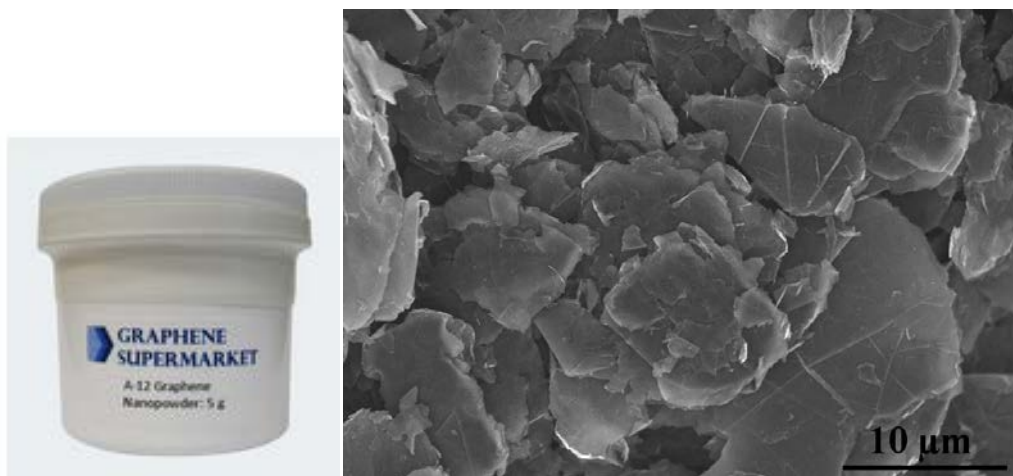
Figure 18: Unmodified Graphene Nanoflakes Obtained from Graphene Supermarket
