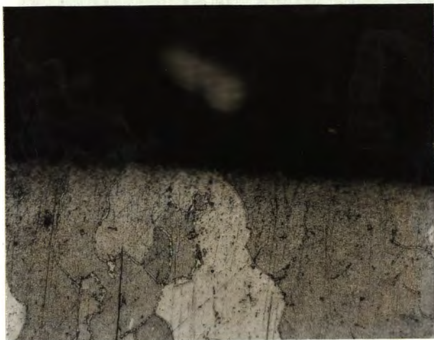
FIGURE 1. LIGHTLY OXIDIZED TURBINE BLADE SURFACE. MAGNIFIED 250X. ETCHED.
