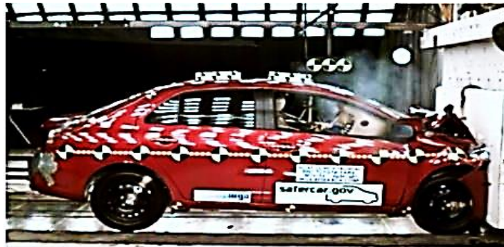
Figure 1.9: Full Frontal Rigid Barrier Impact Test [13]
