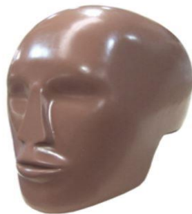
Figure 2.4: Free-Motion Headform Physical Dummy Head [33]
