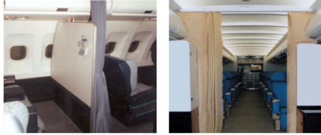
Figure 1.3: Lateral Class Dividers and Aircraft Interiors [6]
