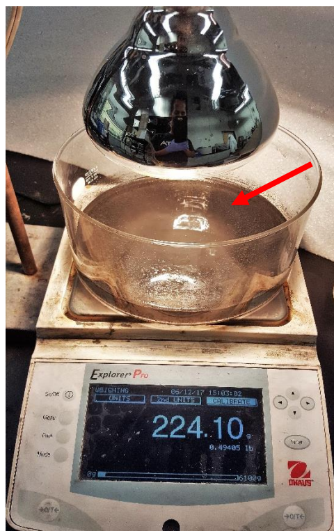
Figure 36. Experimental setup for evaporation with nanoparticles and black base
