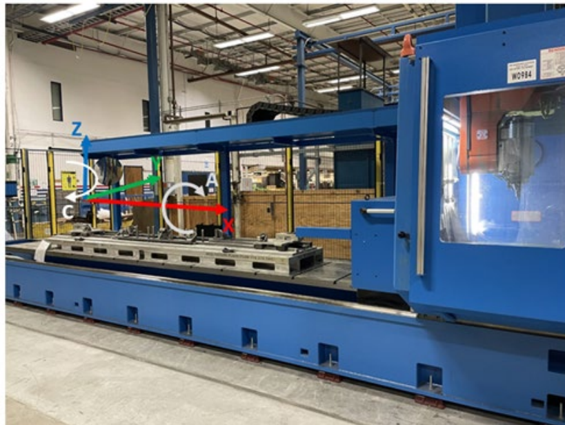
Figure 1. A picture of the Bavius CNC machining center. The machine coordinate system is superimposed on the picture. When the machine rotary axis A = 0°, the spindle is vertical as shown.
