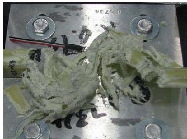
Fig.1 A [\pm 45]_{12} corrugated specimen fractured after crushing.
