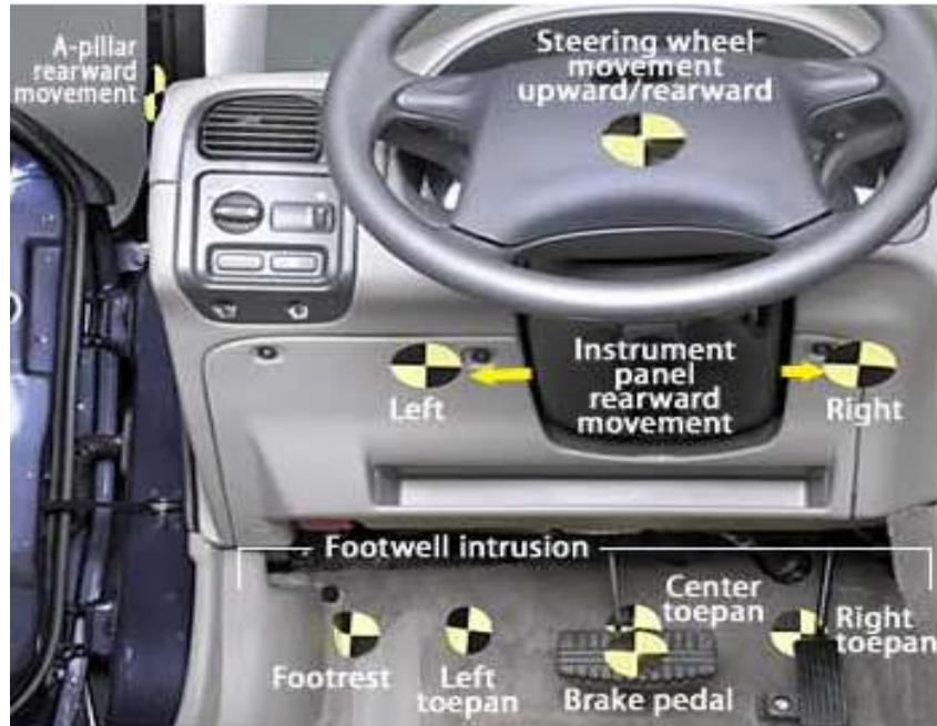
Figure 4.2: US IIHS intrusion measurement locations [20]
