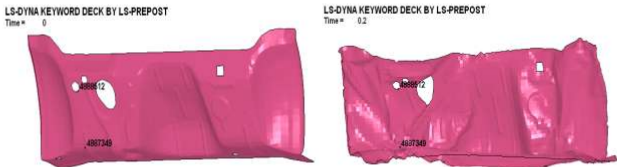
(a): Intrusion in Foot-well of Caravan in CASE-II (isometric view)
