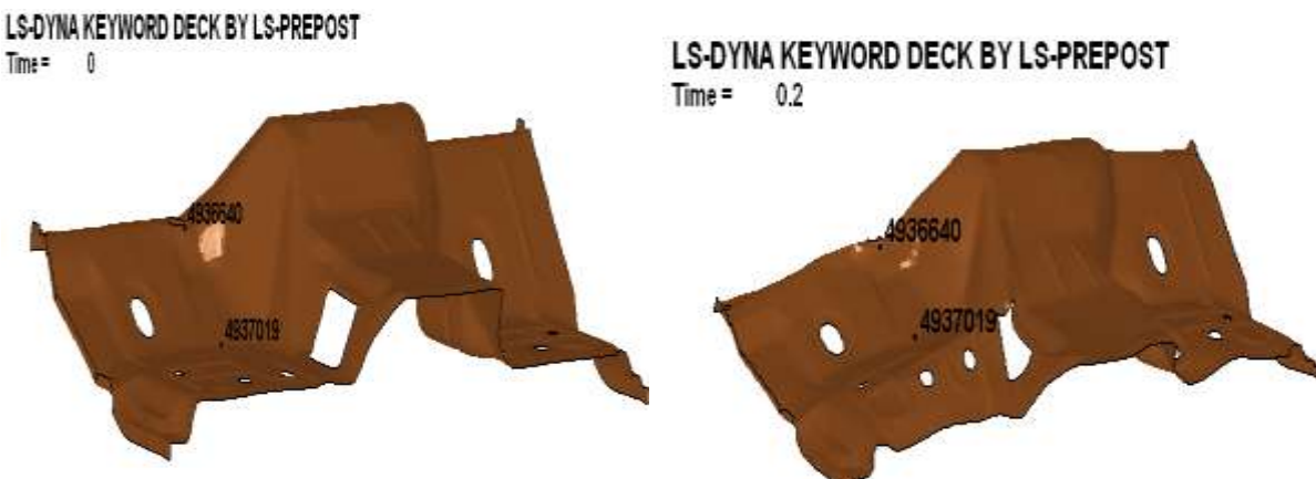
(a): Intrusion in foot-well of F250 in CASE-IV (isometric view)
