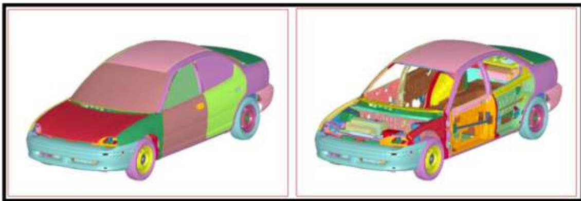
Figure 5.1: Explored view of Dodge Neon FE model [15]
