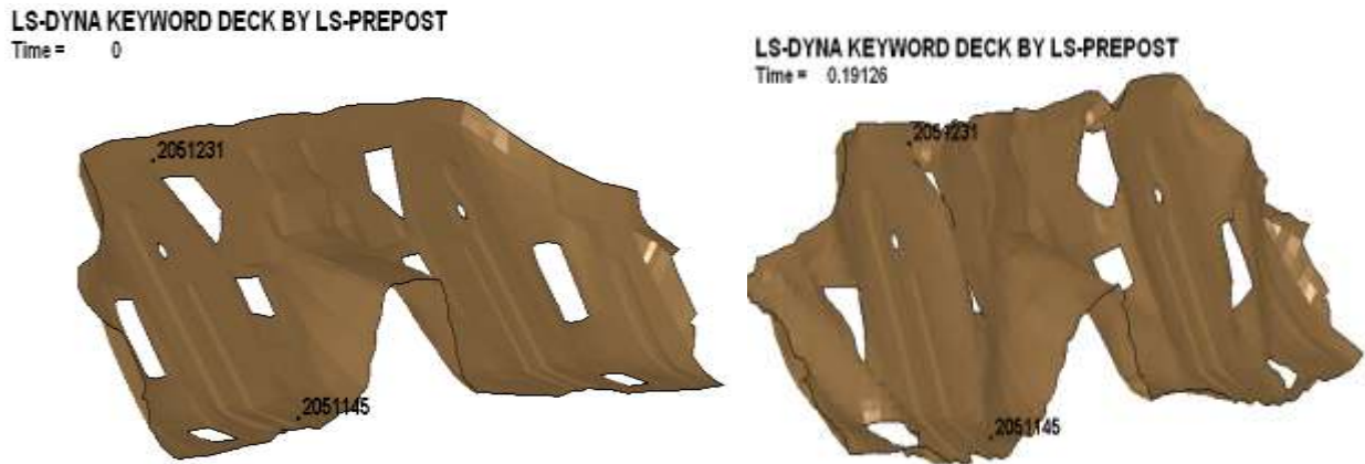
(a): Intrusion in firewall of Rav4 in CASE-VI (isometric view)
