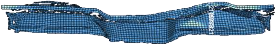
Figure 5.34: Animation sequence showing intrusion in firewall of Explorer in CASE-III
