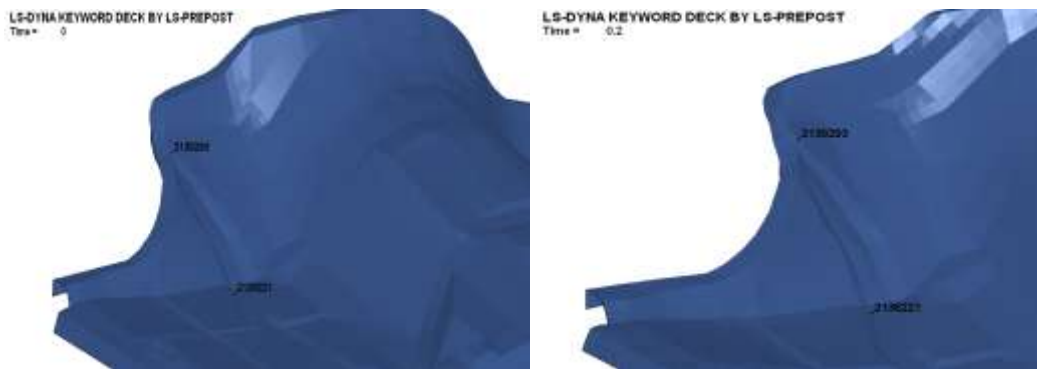
(a): Foot-well intrusion of Chevy S10 in Case-I (isometric view)
