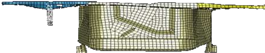
Figure 5.64: Animation sequence showing intrusion in firewall of Ecoline in CASE-V
