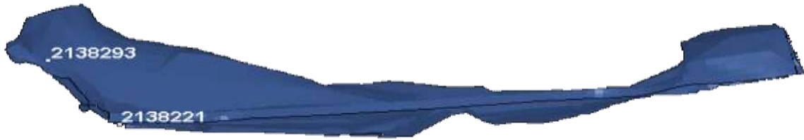
(b): Foot-well intrusion of Chevy S10 in Case-I (side view)
