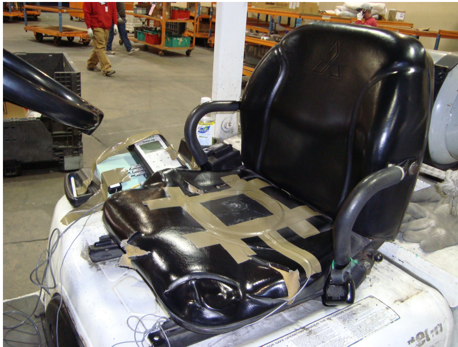
Figure 3.5: Experimental set up with an accelerometer mounted with a seat pad.
