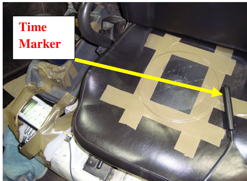
Figure 3.4: Time marker attached to the datalogger.
