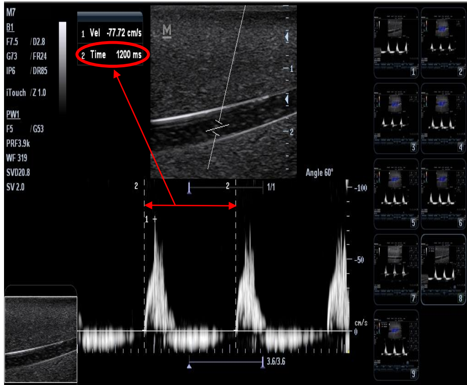
Figure 4.10: Ultrasound image of pulsatile arterial blood flow on arm phantom
