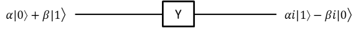
Figure 1.3 The circuit diagram of the Y gate applied on an arbitrary qubit, \alpha|0\rangle + \beta|1\rangle
