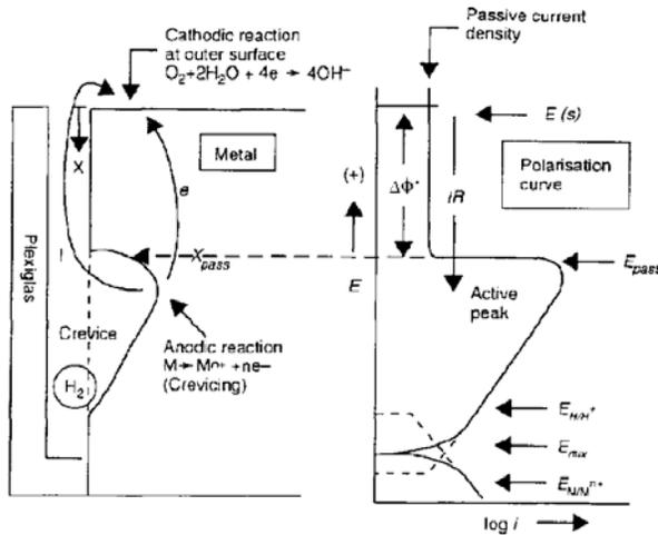
Fig1: Mechanism of active and passive corrosion and its corresponding Anodic and Cathodic reactions in crevice corrosion[3]
