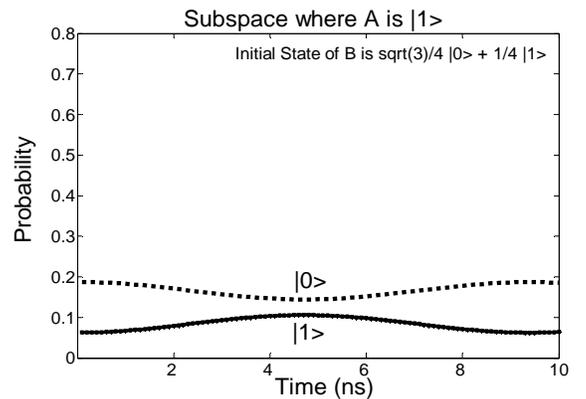
Fig. 4. Evolution of the probabilities of the states  $|0\rangle$  and  $|1\rangle$  of qubit B in the subspace where qubit A is in the  $|1\rangle$  state.
