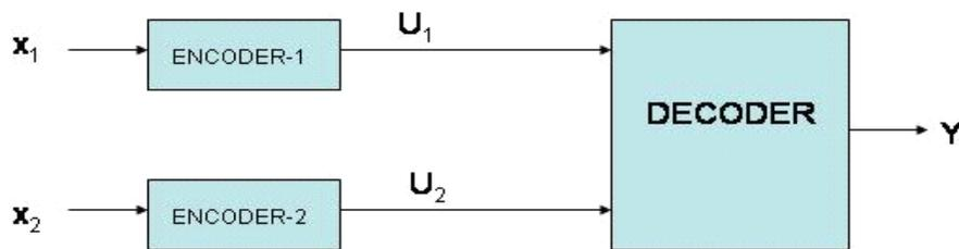
Figure 1: Two sensors sending correlated information to a common destination
