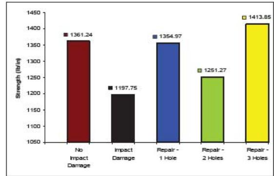
Figure (4): Comparison of Strengths
