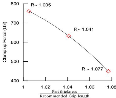
Figure (3): Installation clamp-up force vs. grip ratio
