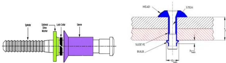
Figure (1): Huckmax® Blind Fastener and a typical blind fastener joint
