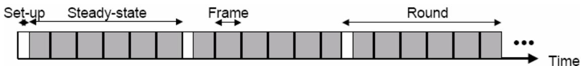
**Figure 4.1.1 Time line diagram of LEACH operation**
