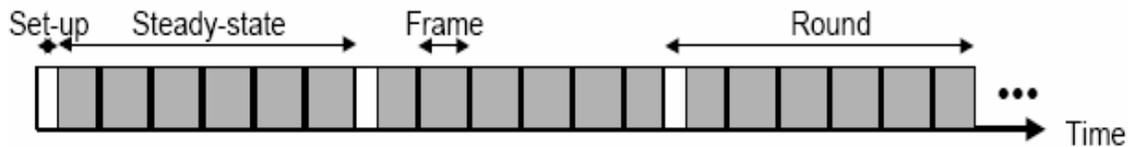
**Figure 2.4.1** Time-line of two phases in LEACH operation. Adaptive clusters are formed during the set-up phase and data transfers occur during the steady-state phase.
