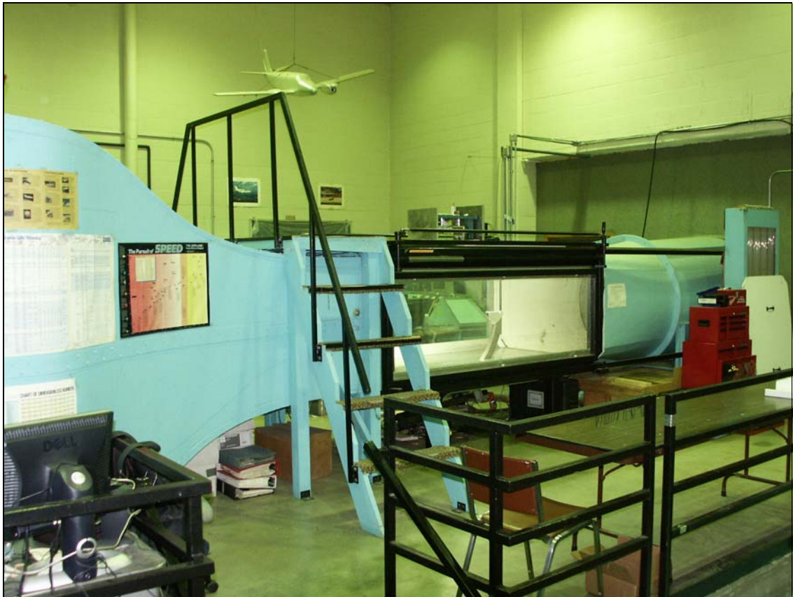
Figure 2: The 3'x4' Low Speed Wind Tunnel, WSU
