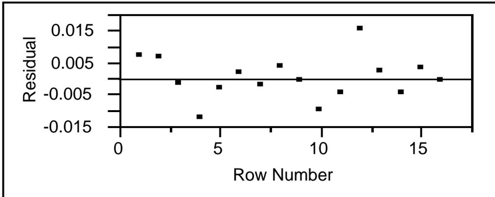
Both residuals versus predicted and residual versus run order plots appear to be random with no significant pattern the experimental error is normally independently distributed.
