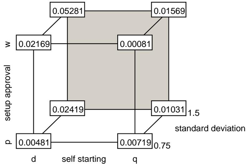
We can see from the cube plot that Joint monitoring scheme with Dynamic EWMA (d) and precontrol setup approval scheme (p) produce lowest MSE (Mean squared error) for low standard deviation .75.
