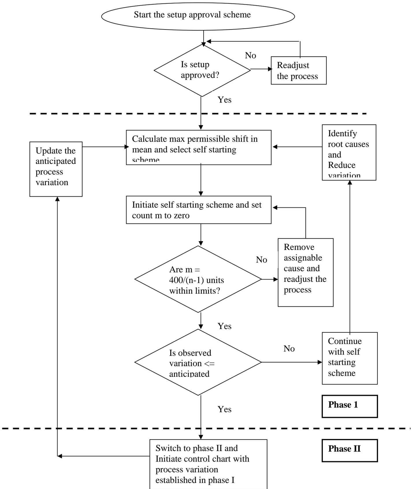
Fig 11. Proposed joint monitoring scheme
