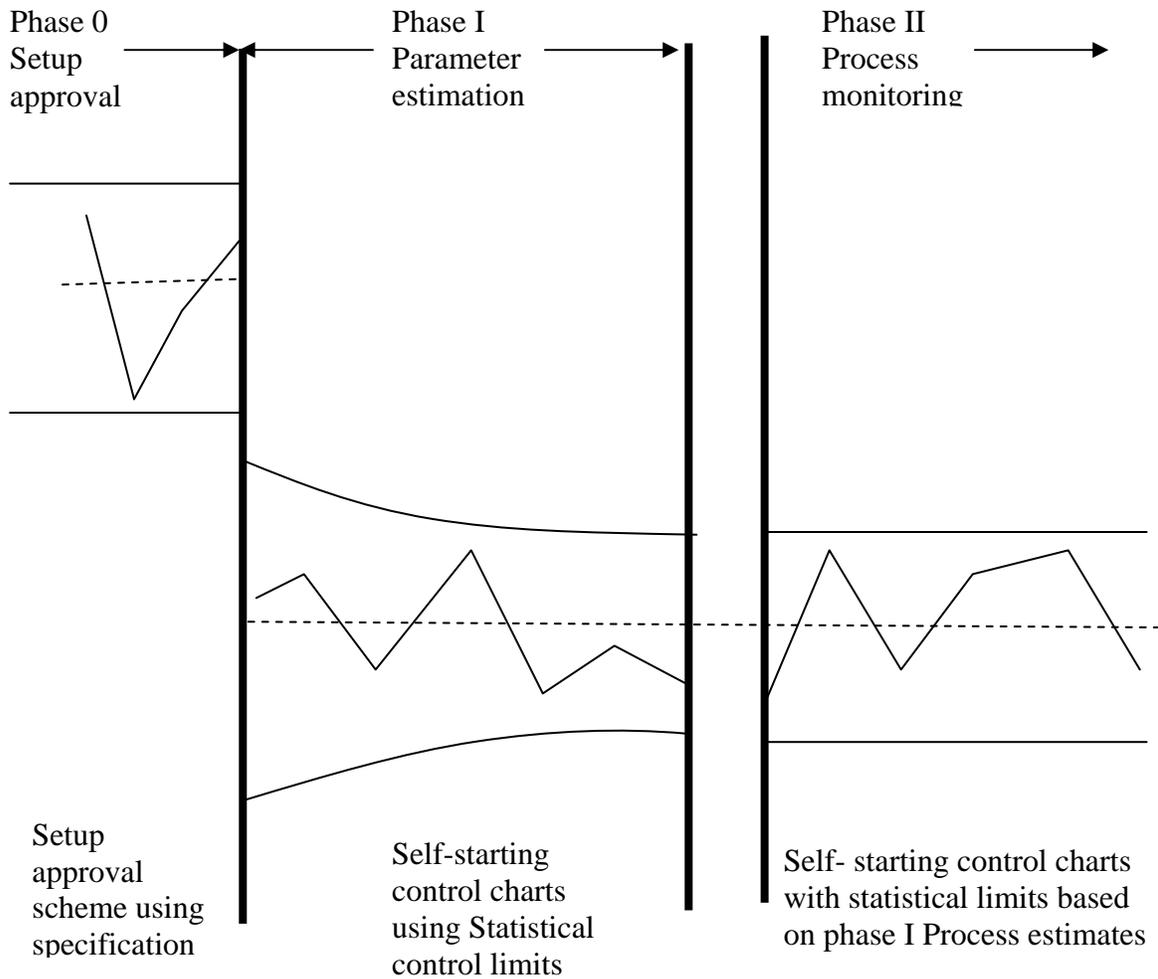
Fig. 9. Scenario for Joint monitoring scheme where anticipated capability is verified and process is stable
