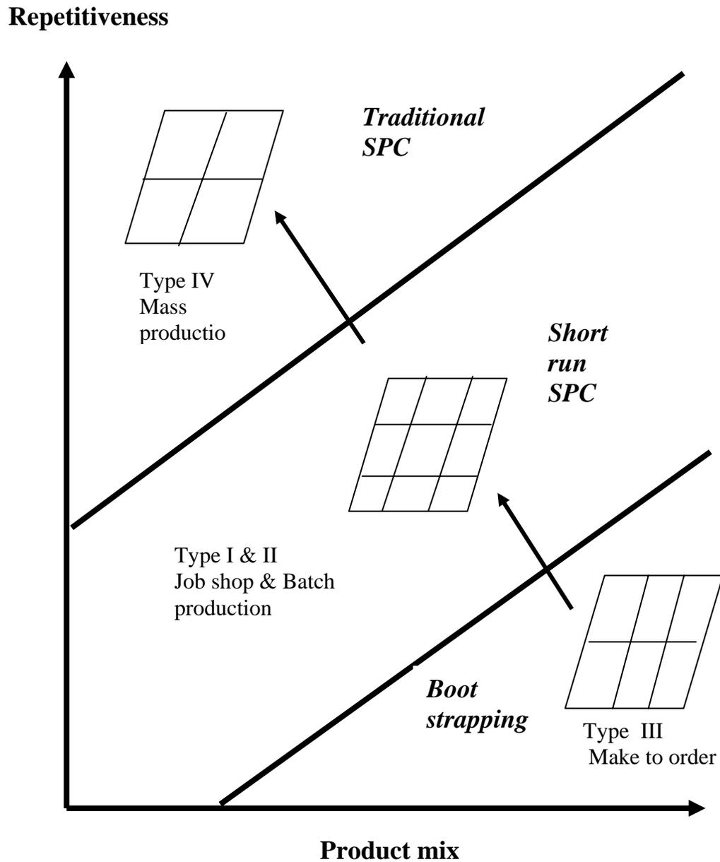
Fig 7. Application of SPC for different types of production processes
