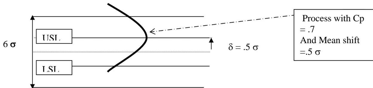
Fig 16 Process with CP .7 and mean shift .5 Sigma
