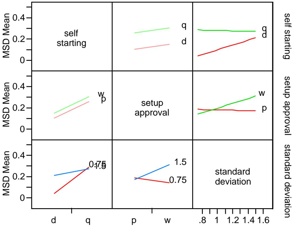
From the interaction plots between self starting scheme and standard deviation we can clearly see that d (Dynamic EWMA) is better than q (Q chart) for low standard deviation of .75.
