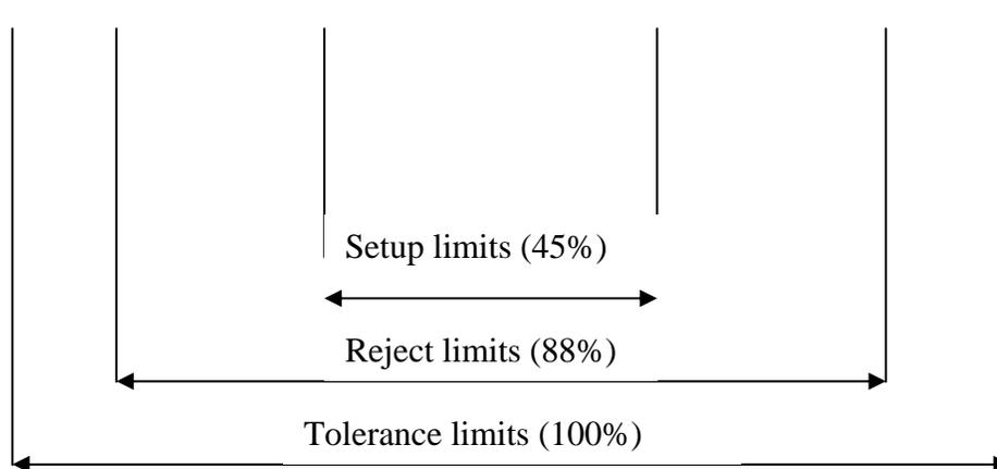
**Fig. 4 Nomogram for setup limits proposed by Feigenbaum**
