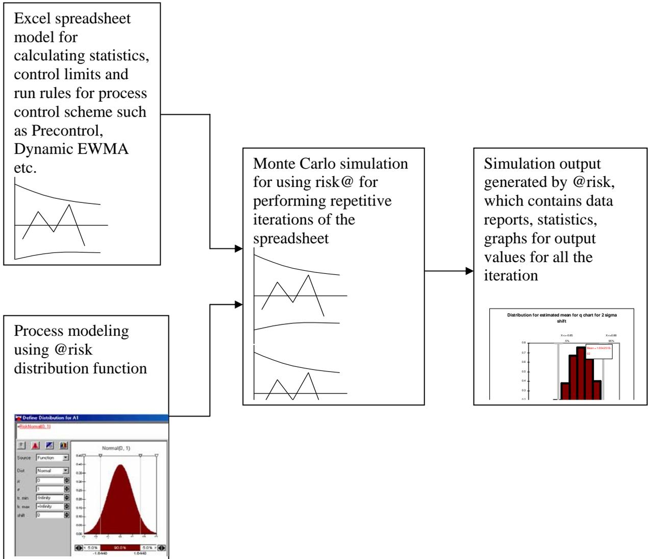
Fig. 12 Simulation methodology for comparing different process control techniques
