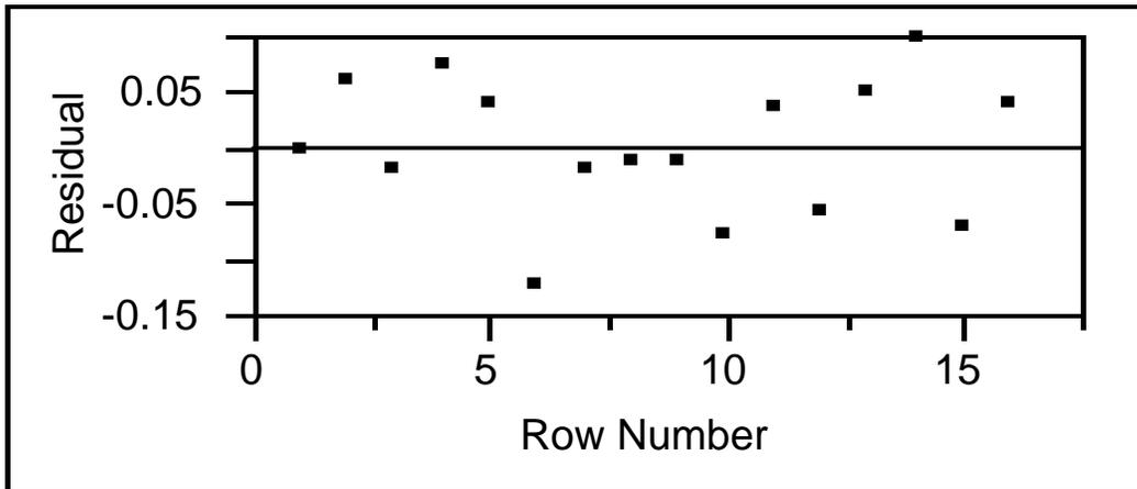
Both residuals versus predicted and residual versus run order plots appear to be random with no significant pattern the experimental error is normally independently distributed.
