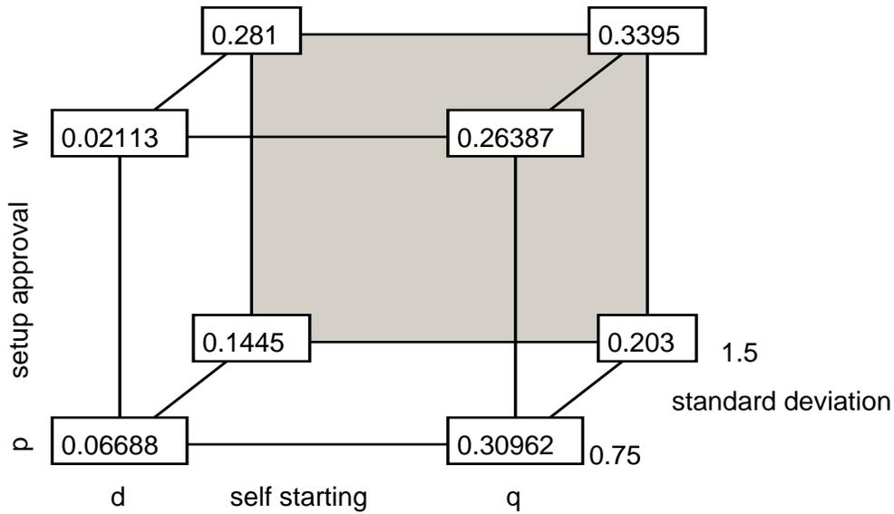
We can see from the cube plot that Joint monitoring scheme with Dynamic EWMA (d) and Wheeler setup approval scheme (w) produce lowest MSD (Mean squared deviation) for low standard deviation of .75.
