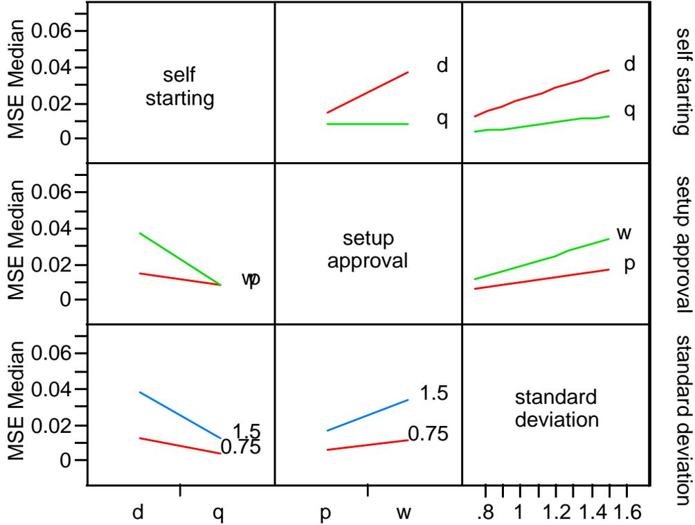
From the interaction plots between self-starting scheme and setup approval scheme we can clearly see that MSE for d (Dynamic EWMA) is similar to q (Q chart) for if we use Precontrol setup approval schemes. But MSE for d (Dynamic EWMA) is much higher than q (Q chart) for if we use wheeler setup approval
