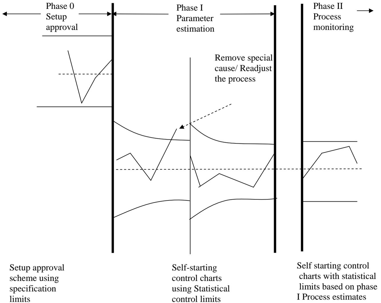
Fig. 10 Scenario for joint monitoring scheme where anticipated capability is verified process was unstable
