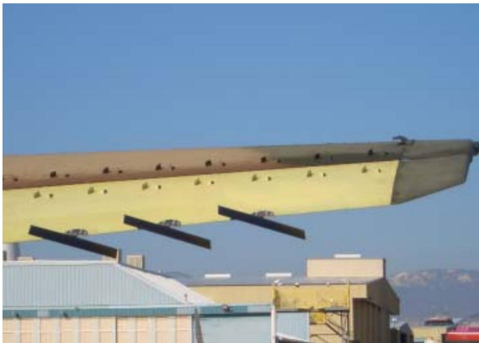
Figure A-8. Aileron Tabs installed on Bosbok
