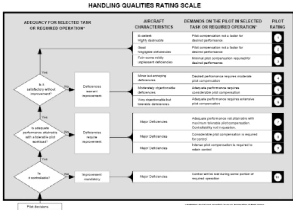
Figure A-10. Cooper-Harper rating scale [5].
