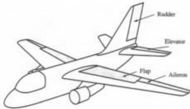
Figure A-1. Normal airplane configuration.
