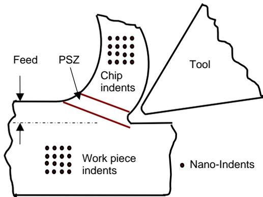
Figure 3: Schematic shows the location of indents on the chip and on the workpiece
