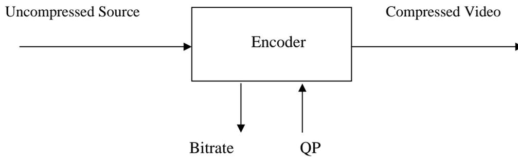
**Figure 4.3: Open Loop Encoding (VBR)**
