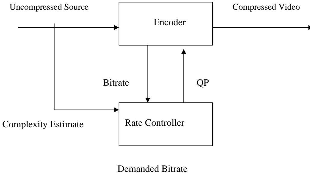
**Figure 4.4: Closed Loop Rate Control (CBR)**
