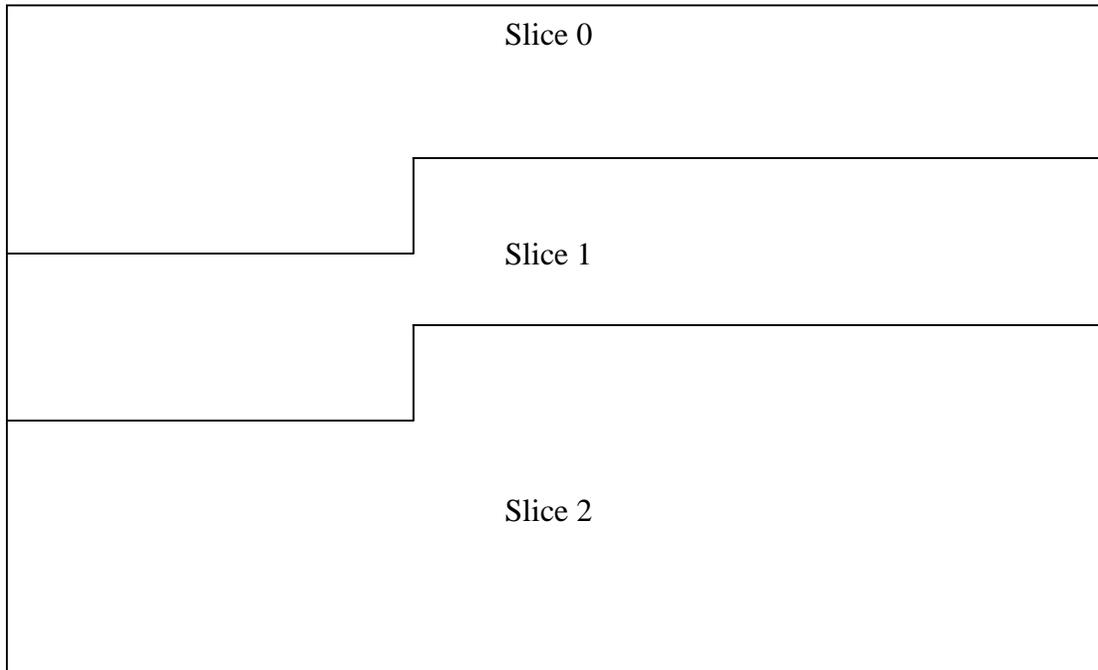
**Figure 2.3: Partitioning of picture into slices**
