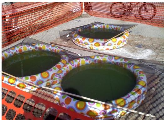
Figure 1: Three open-ponds (100L, 10-cm deep) using inflatable kids pool
