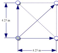
Fig. 1. Piezoelectric disk placement. Each sensor would pulse a signal to the remaining three through the material.
