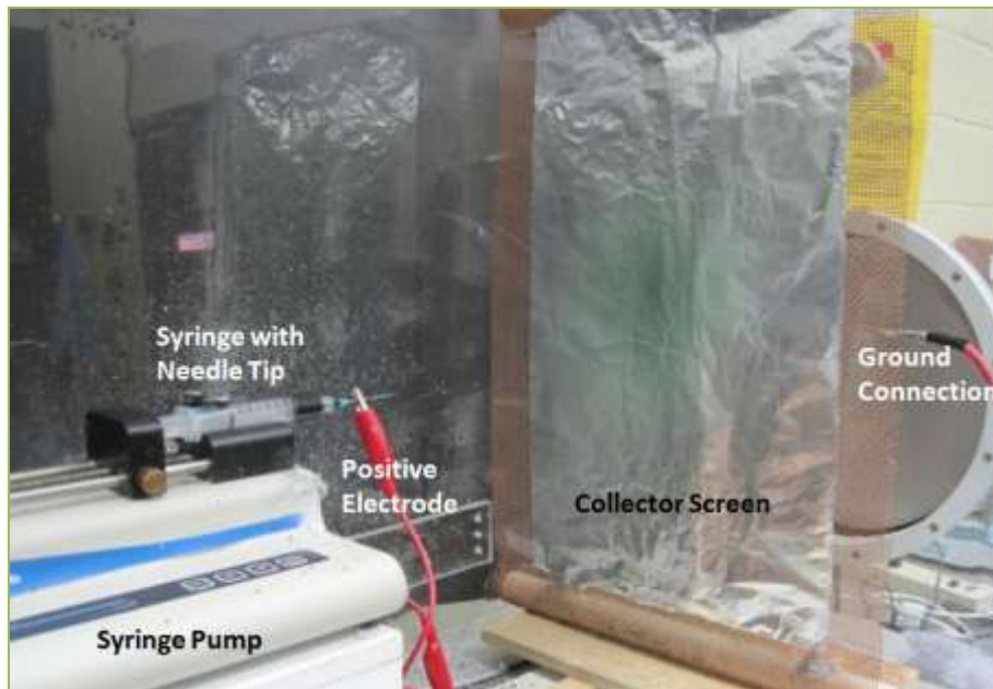
Figure 10. Digital image of the setup used for electrospinning.
