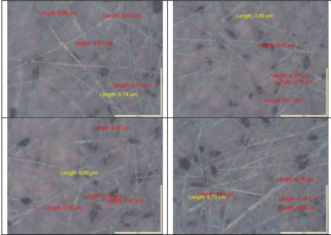
Figure 1: Microscopic images of fibers taken at 4 random locations when the fiber was electrospun at 0.5 ml/hr flow rate
