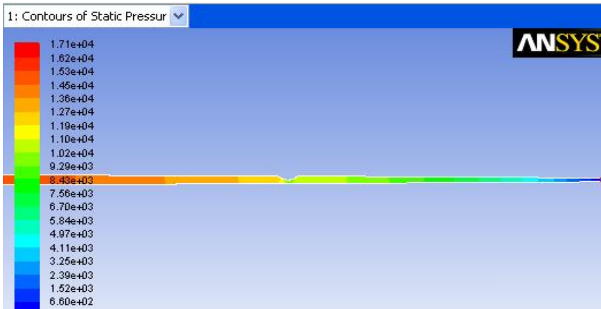
5-2 Contours of Pressure for Fifty Percent Blockage
