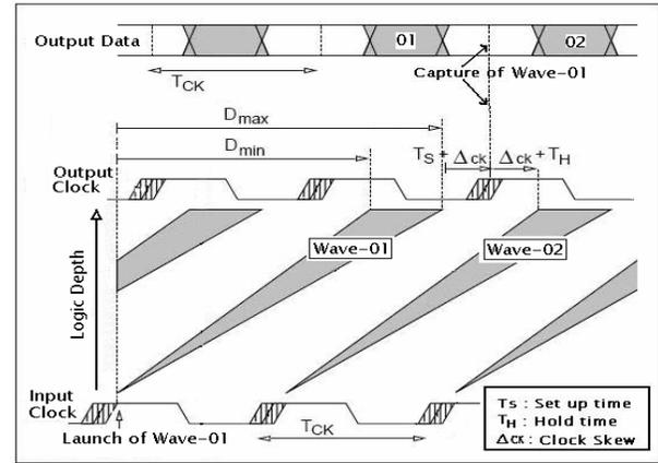
Fig. 2. Spatial diagram for wave pipelining showing delay contours
