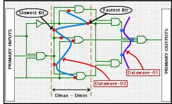
Fig. 1. A random circuit showing data bits with different speeds
