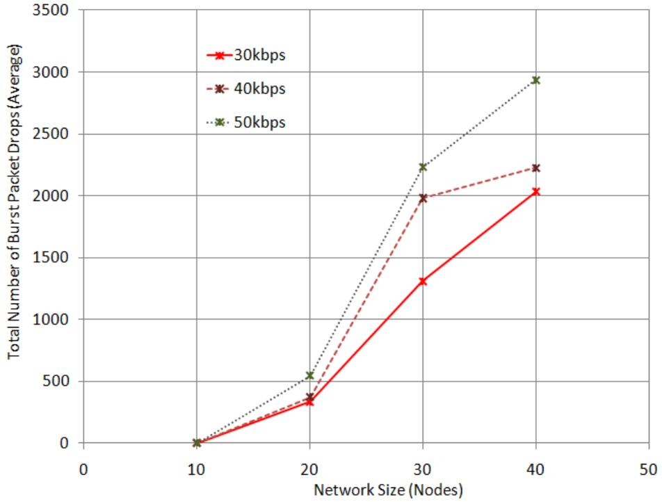
Figure4. Network Size Vs Burst Packet Drop (Average) in Stationary Network
