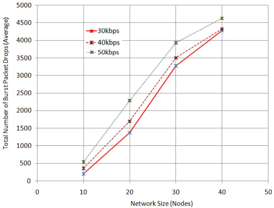
Figure5. Network Size Vs Burst Packet Drop (Average) in Mobile Network
