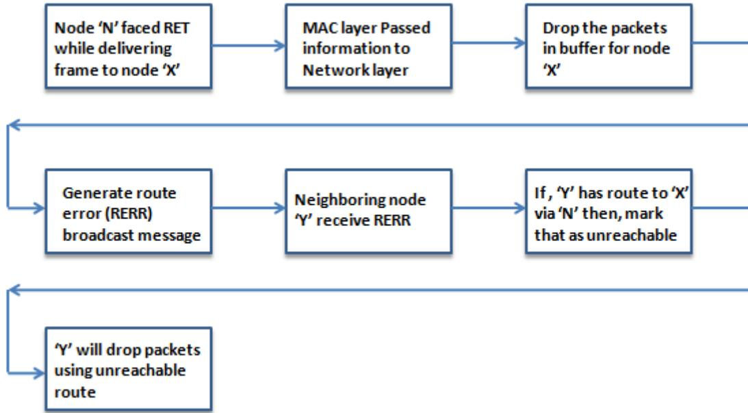
Figure 5: Burst Loss Occurrence (Node 'N' faced RET issue, MAC layer of node 'N' passed information to the network layer which will drop packets in the queue waiting to be transmitted to the next-hop node 'X' and will broadcast RERR message. Node 'Y' upon reception of RERR will mark the route passing through 'N' for destination 'X' as unreachable and will drop its packet in the queue for node 'X' )
