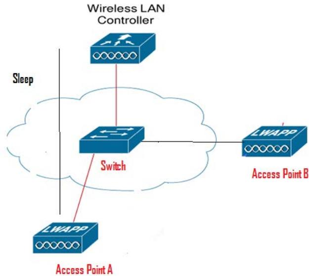
Figure 13: Phase 1. Controller sleeping the access point
