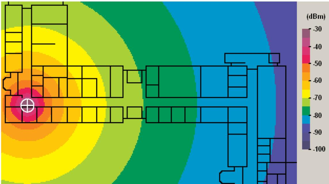
Figure 7: Coverage prediction by one-slope model [7]
