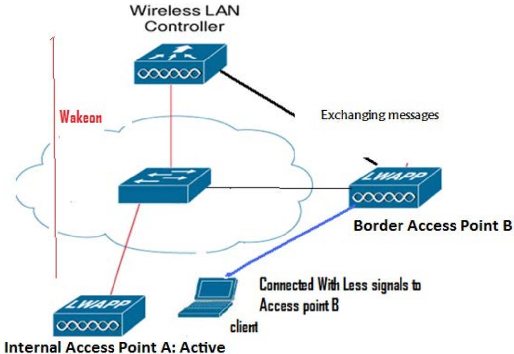
Figure 16: Phase 4. Now-active Access Point A after receiving wake-on WLAN signal from controller
