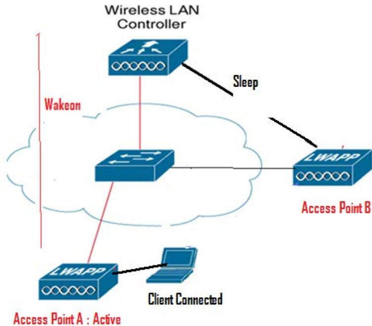
Figure 18: Phase 6. Sleeping Access Point B when no clients are connected
