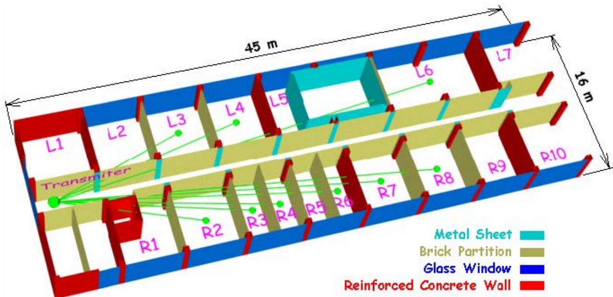
Figure 8: Multiwall model geometry
