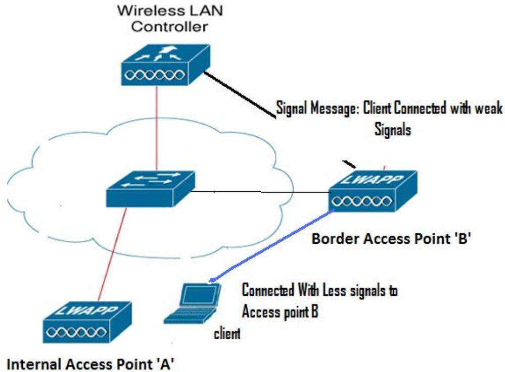
Figure 15: Phase 3: Client in vicinity of sleeping Internal Access Point A but getting connected to Access Point B
