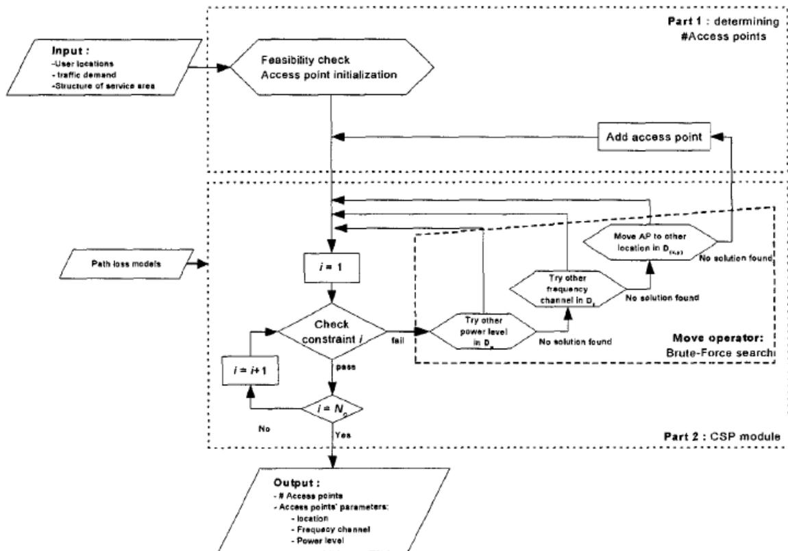
Figure 9: Constraint-based design algorithm [8]
