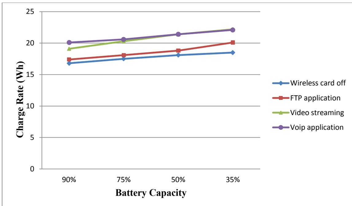
Figure 3.5 Charge rate for each application versus battery capacity
