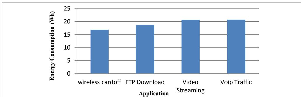
Figure 3.4 Instantaneous energy consumption of each application
