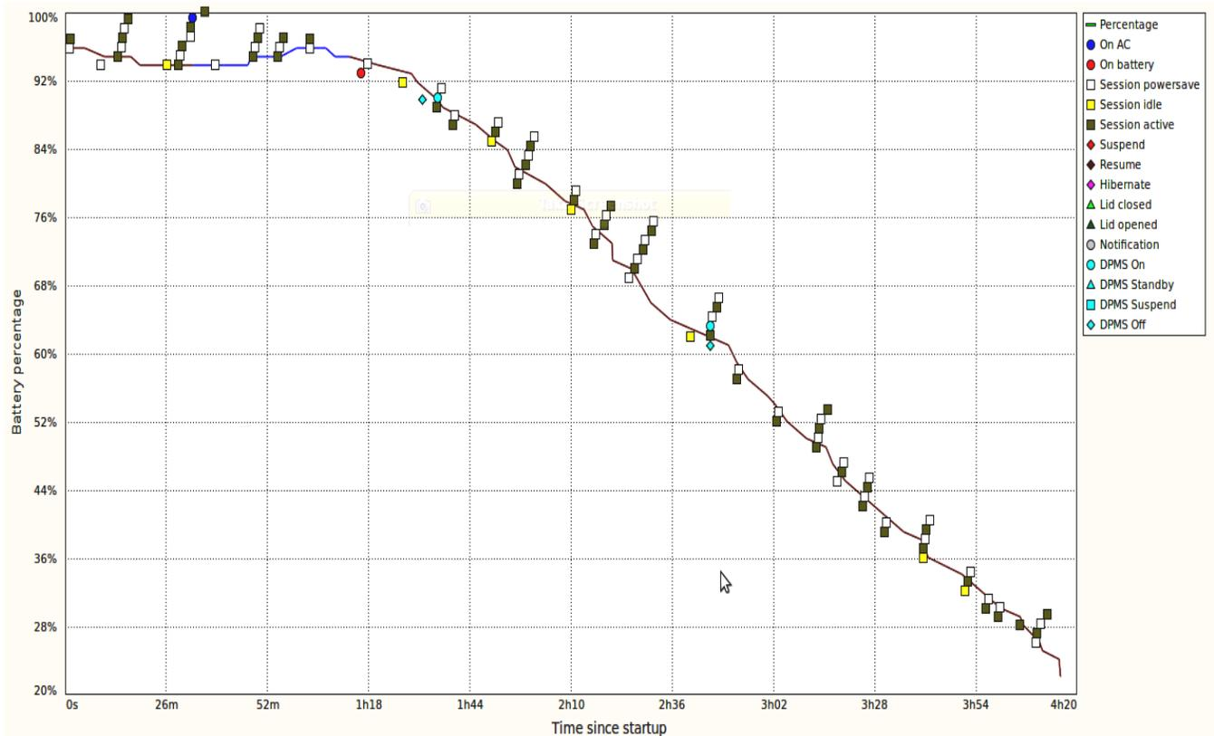
Figure 3.2 Battery discharge versus time since startup
