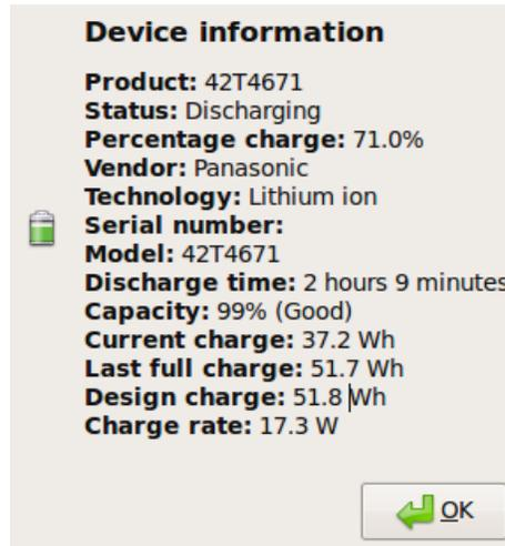
Figure 3.3 Battery device information
