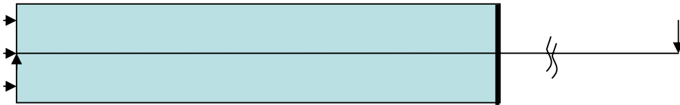
Figure B2. Model with a long arm (dummy beam) used for bending (Sheet length= 50 mm, length of dummy beam = 1500 mm).
