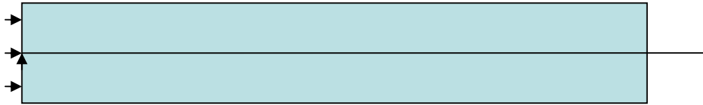
Figure B1. Model with a dummy beam (length of sheet=100 mm; thickness of sheet = 4 mm; length of dummy beam = 110 mm).
