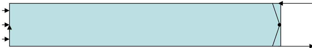
Figure B3. Model used for current study (Length=50 mm, thickness of sheet=4 mm).
