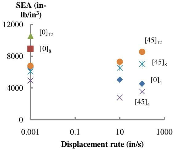
Fig.2: Specific energy absorption for different ply stacking sequence at various loading rates.
