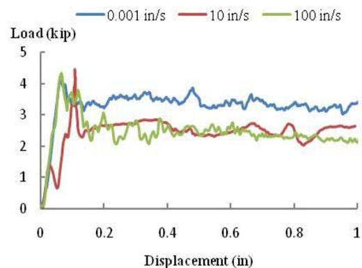
Fig.1: Load-displacement response of  $[0]_4$  E-glass prepreg at various loading rate.
