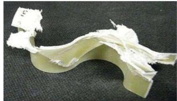
Figure 4: Failure mode of  $[45]_4$
