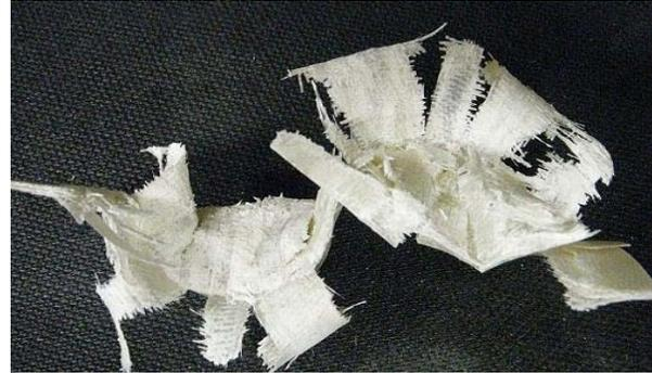
Figure 3: Failure mode of  $[0]_4$
