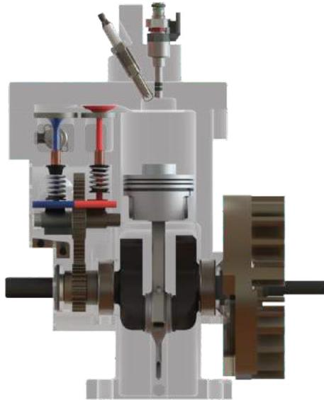
*Figure 8 Nautilus GEN III engine design (Davani, 2019)*
