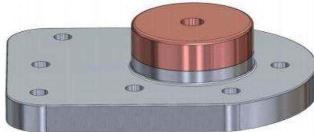
*Figure 6 Primary combustion chamber with copper glow plug in the middle. (Davani, 2019)*
