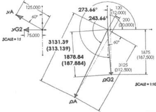
Figure 7. Crank velocity polygon and acceleration polygon
