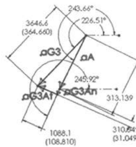
Figure 10. Coupler acceleration polygon for acceleration of the center of mass
