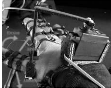
Figure 2. Stage 3 Prototype thumb abduction, adduction, and flexion
