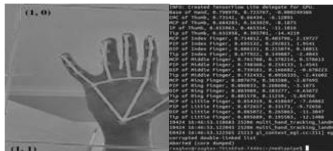
Figure 3. Normalization of coordinates for keypoint estimation and coordinate output
