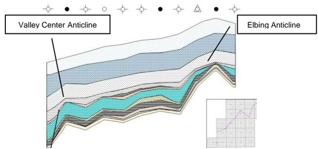
Figure 3. Cross sectional view of present day structure across the study area from the southwest to the northeast. The Valley Center and Elbing anticlines can be seen, as well as normal faulting to the west of the Valley Center anticline.
