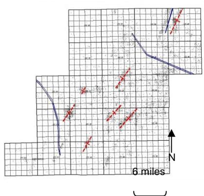
Fig. 2 Map of structural trends in the study area. Northeast trending dashed lines indicate anticlinal structures. Fault zones are indicated by solid lines.
