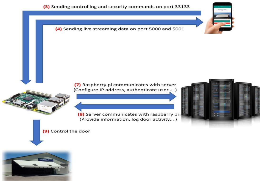
Figure 6. Communication between Raspberry Pi, application, central server, and door relay
